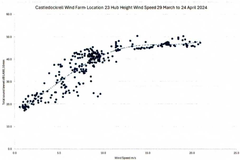
Figure 11-4 Measured Noise Levels NML2 – Property 23 – Hub Height
