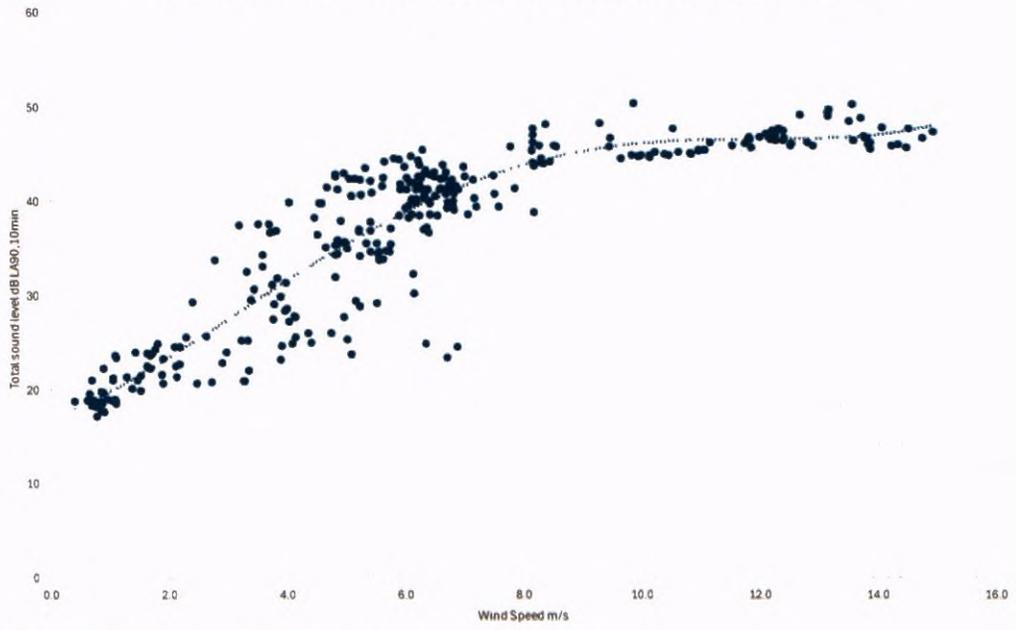
Figure 11-5 Measured Noise Levels NML2 – Property 23 – 10m Height
