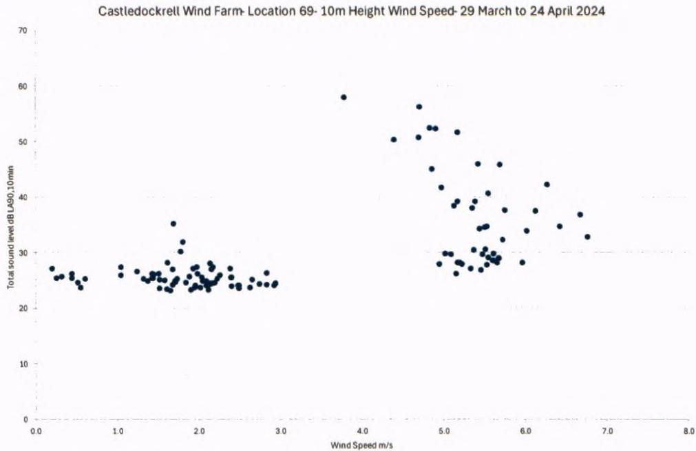
Figure 11-3 Measured Noise Levels NML1 – 10m Height
