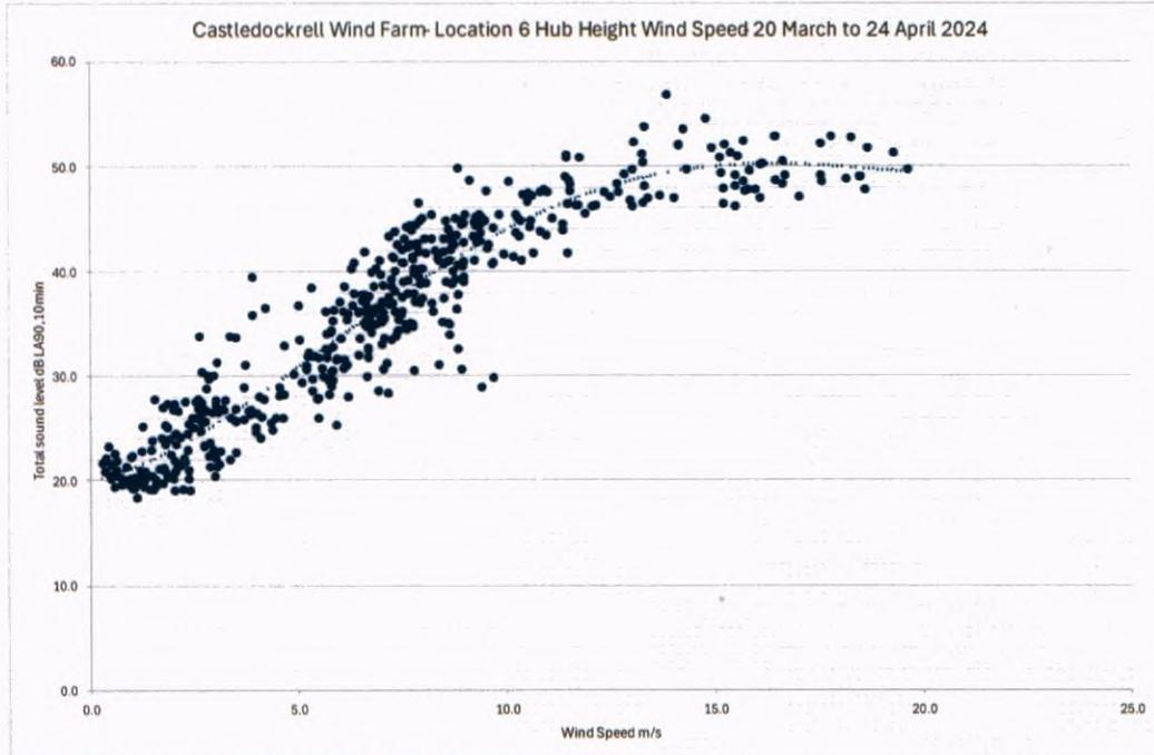
Figure 11-8 Measured Noise Levels NML4 – Property 6 – Hub Height
