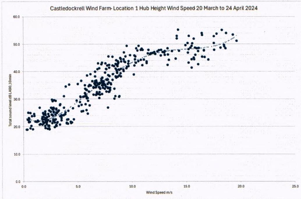
Figure 11-6 Measured Noise Levels NML3 – Property 1 – Hub Height
