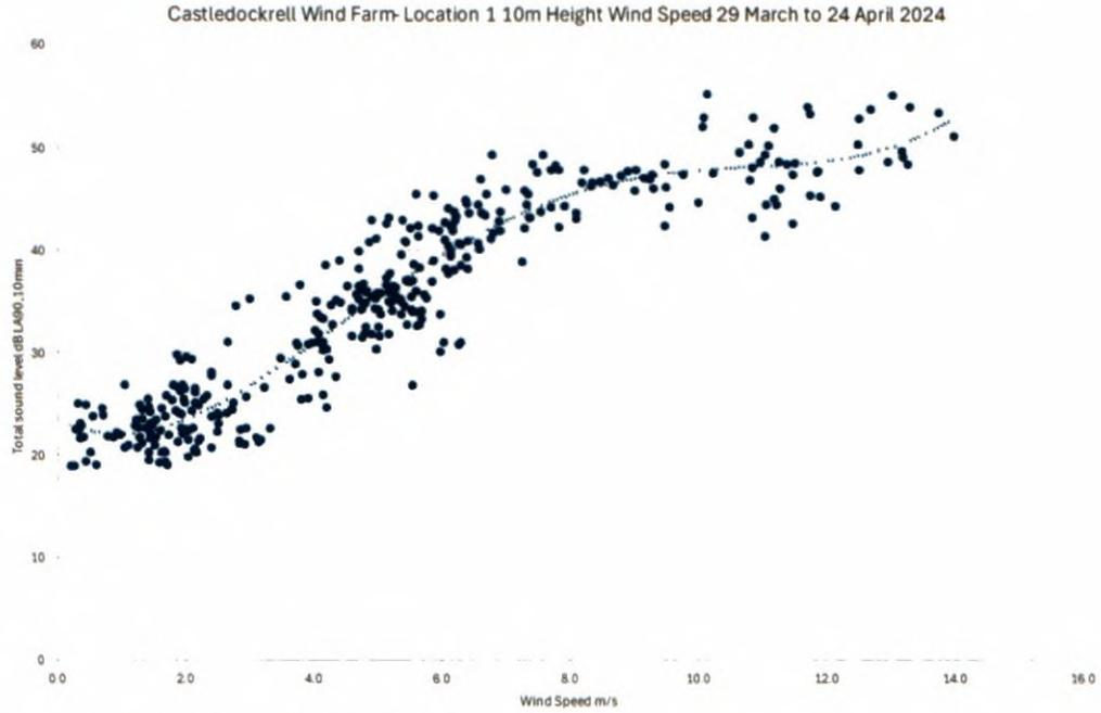
Figure 11-7 Measured Noise Levels NML3 – Property 1 – 10m Height
