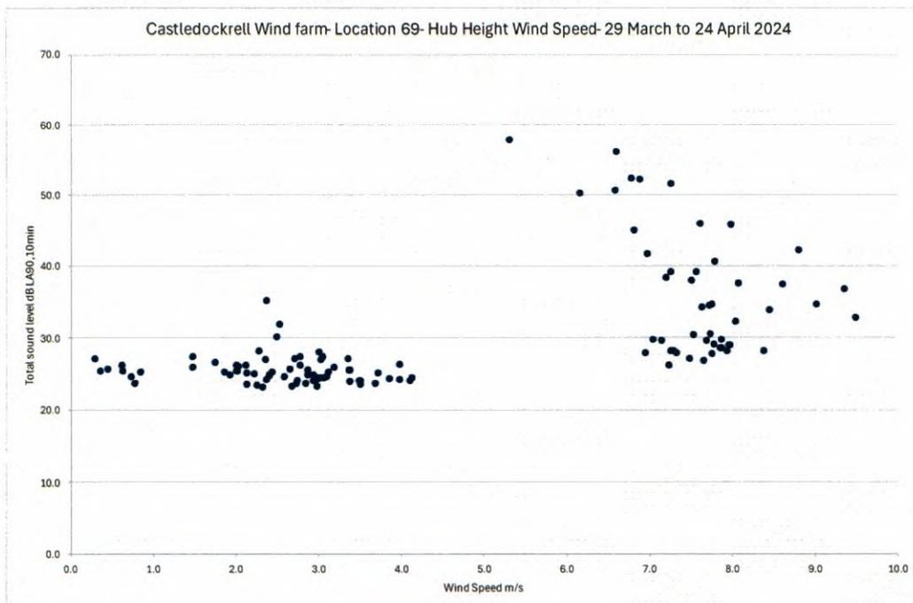
Figure 11-2 Measured Noise Levels NML1 – Hub Height
